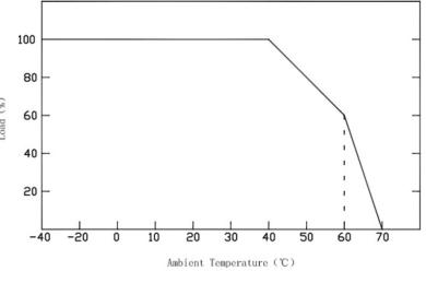
If being used in higher ambient temperatures, ensure the load on the LED driver is de-rated in accordance with this chart. Failure to do so could lead to a failure, which is not covered by the warranty
