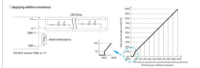
Note: 1. Min. duty cycle of output current is about 1%, and the dimming input is about 6KΩ or 0.6VDC, or 10V PWM signal with 6% duty cycle.
