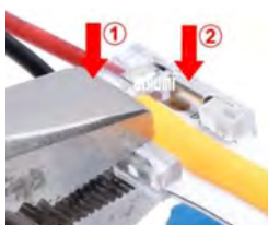
3. Clamp metal teeth to pierce PCB one by one
